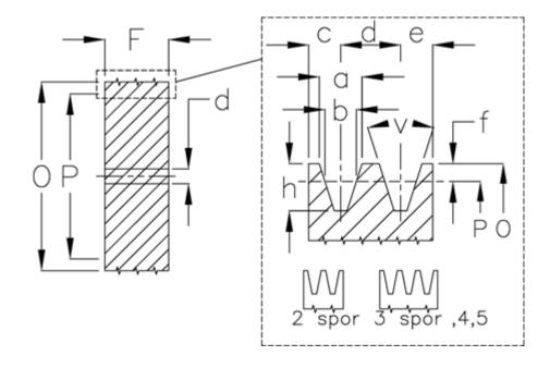
$\begin{array}{ll} d & = 15 \\ F & = 80.0 \\ Number of ribs = 5 \\ O & = 85.5 \\ P & = 80 \\ Type & = A \end{array}$
